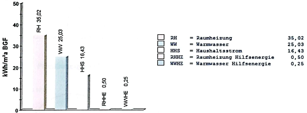
Energiebedarf in kWh/m 2 a BGF
